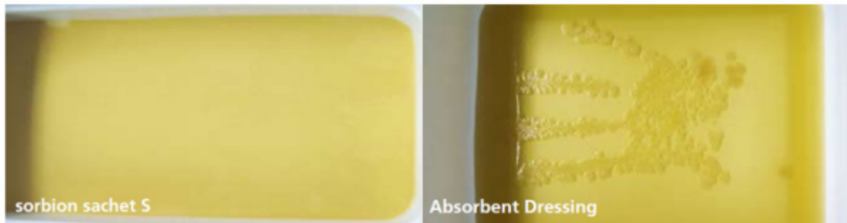
Figure 1: Qualitative demonstration of an in vitro experiment on absorbing pathogens. sorbion sachet S and another absorbent dressing were exposed to a solution containing 10^4 CFU/ml Staphylococcus aureus subsp. aureus Rosenbach, Gentamicin- and Methicillin-resistant, (ATCC 33592, [13]) and then pressed with a gloved hand. Immediately thereafter an impression of the glove was taken on an agar plate and incubated for 48 hours at 37 °C [9].
