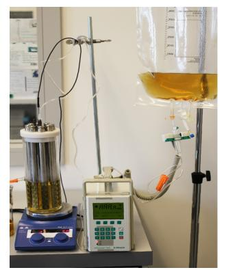
Figure 1: Experimental setup. On the left European Biofilm Reactor (EUREBI) with vertical placed titanium discs, on the right infusion bag as storage vessel for liquid culture, in the middle Infusomat to control the flow of liquid culture.
